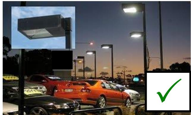
Full cut-off box lights direct light downwards and are cheaper to operate
