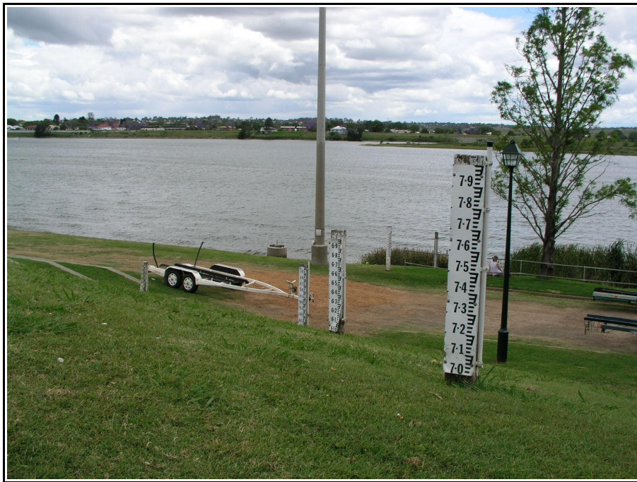
Figure 3.26 Flood Markers, Prince Street
