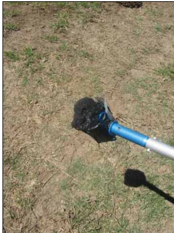
Figure 5: The sediment sampling device, showing some sediment collected from one of the drains.
