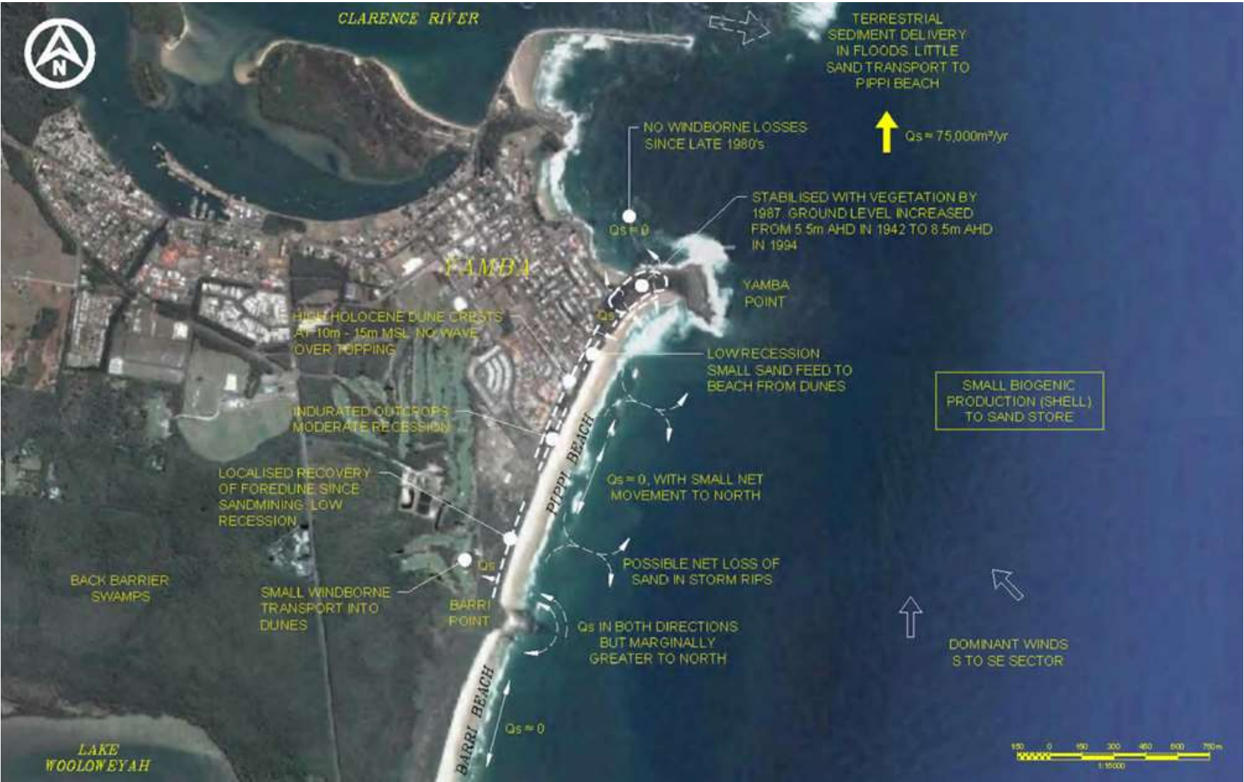
Figure 24: Conceptual model of sediment processes at Pippi Beach
