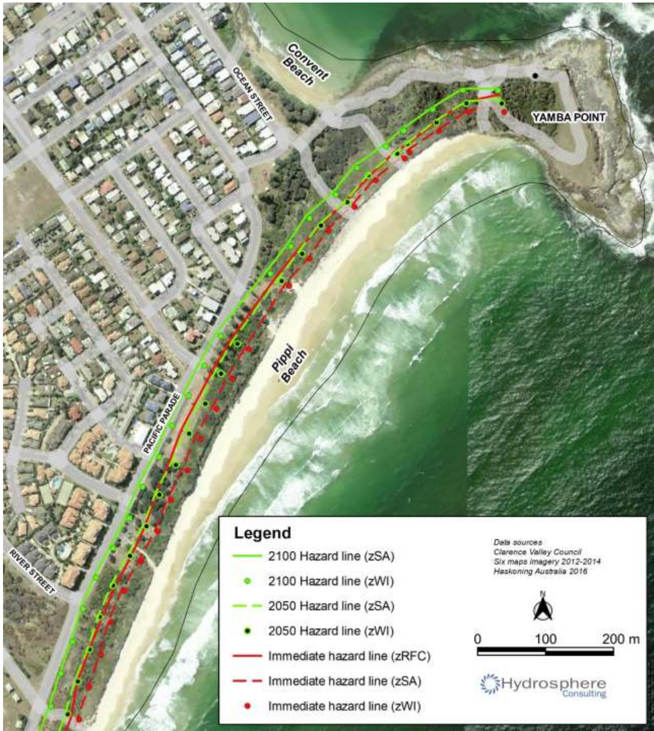
Figure 25: Coastal hazard lines for Pippi Beach - north
