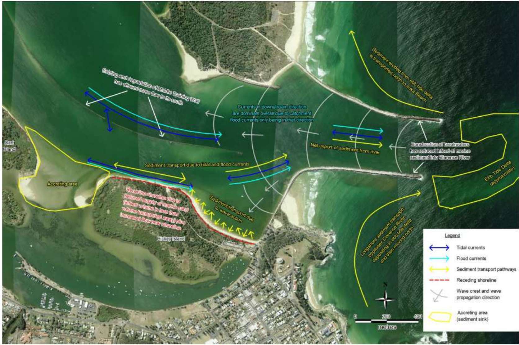
Figure 21: Conceptual sediment processes occurring at Whiting Beach
