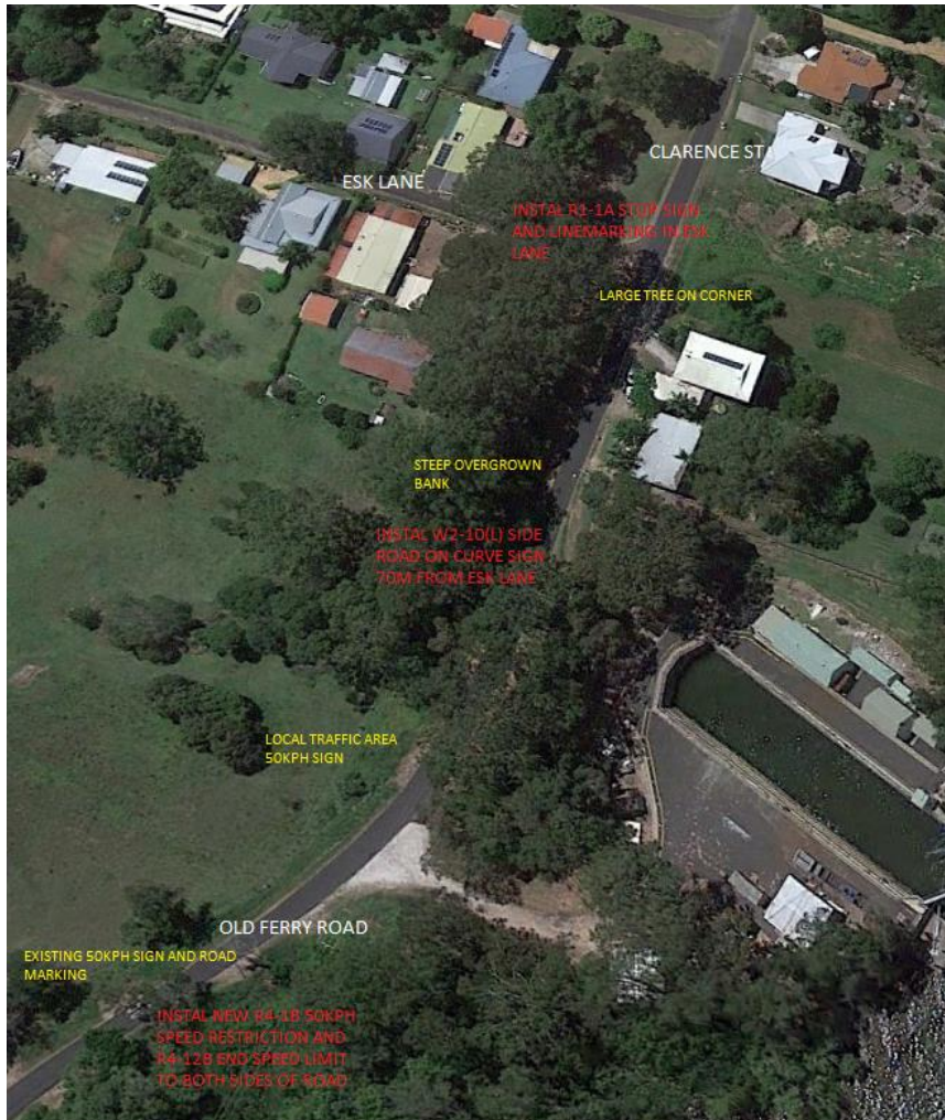
Road Features and Recommended Treatments.
