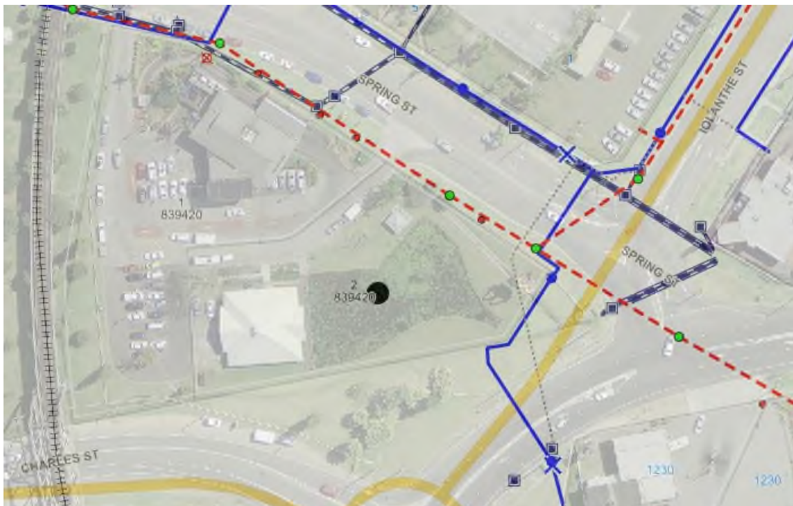
Services - red sewer, blue water, grey stormwater
