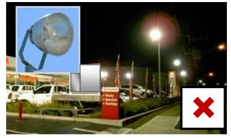
An inefficient light is aimed almost horizontally spilling light upwards and dazzling motorists
