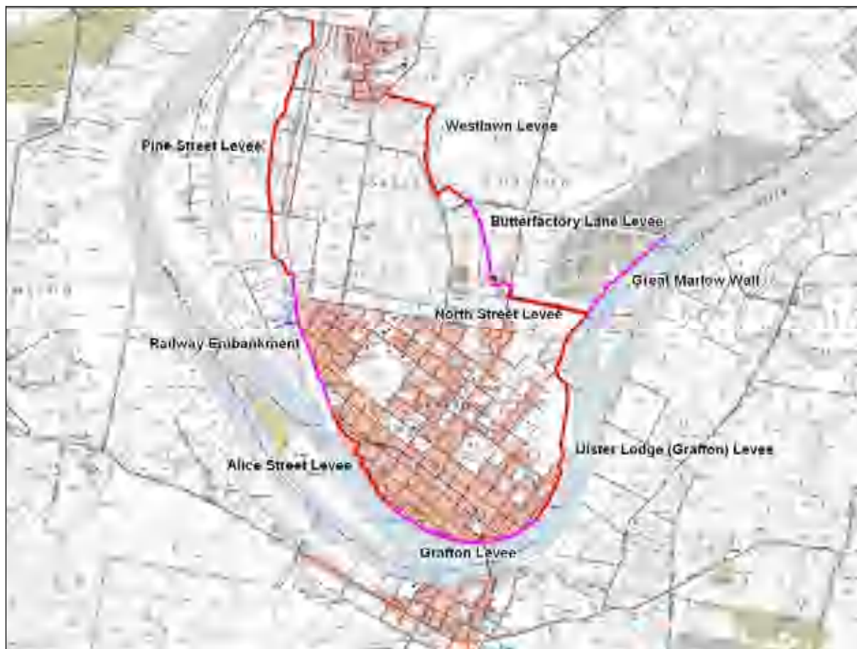
FIGURE 5.1 Grafton Levee System
