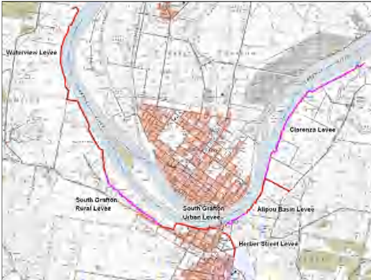
FIGURE 5.4 South Grafton Levee System
