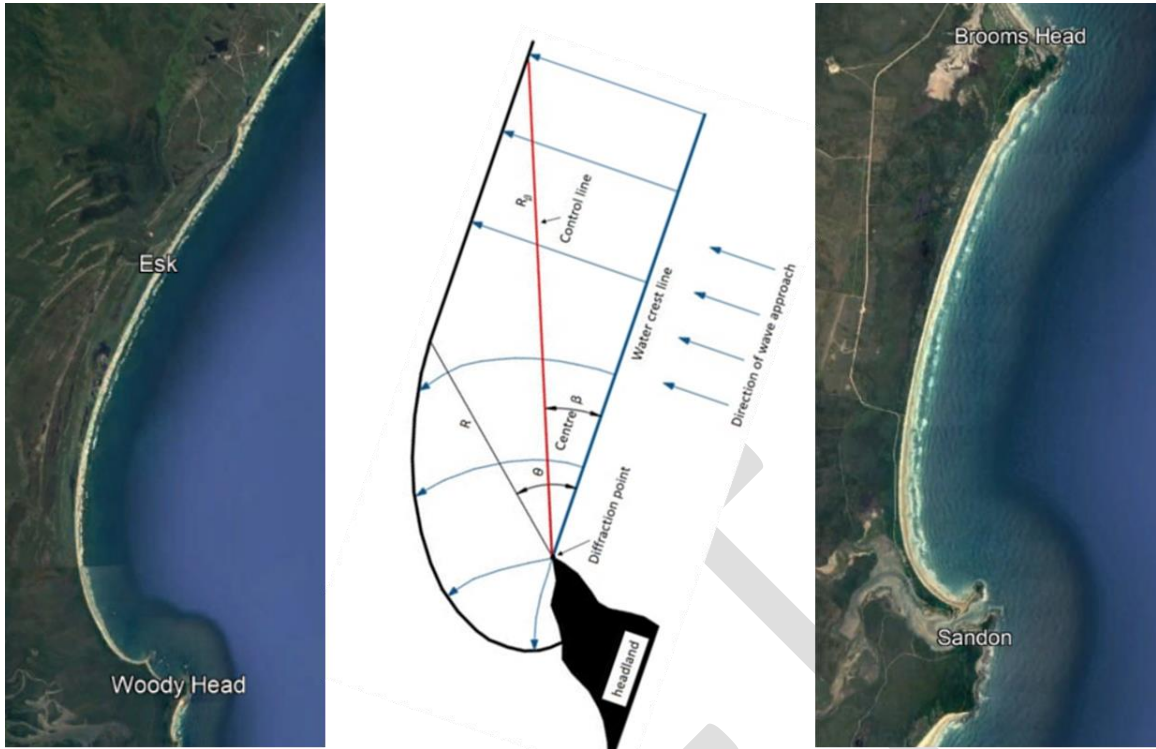
Figure 7-5: Examples of parabolic beaches in the study area, and the Definition sketch for the parabolic equations
