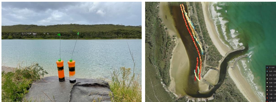
Figure 6-2: Drifters and recorded tidal current velocity
