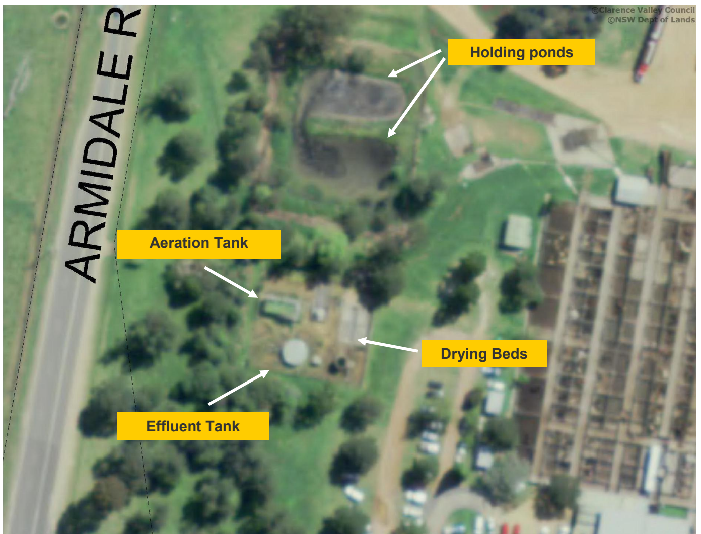
Figure 1 - Grafton Regional Saleyard Treatment Plant Site Plan
